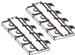
4. Install the disk support back to the NVR.
